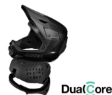
Increased protection with DualCore technology The advanced version of KinetiCore, for more demanding rides. Two different density EPS layers form one helmet. The soft low density layer sits close to the head, protecting you against rotational impact. The hard high density later sits further away from the brain ready to absorb direct impact.
