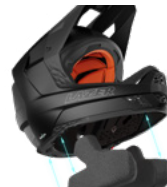
Emergency padding In case of a crash the cheek pads can be pulled out of the bottom of the helmet without having to remove the helmet first. Creating space to carefully remove the helmet, minimising the need to move the head around too much and cause injuries.
